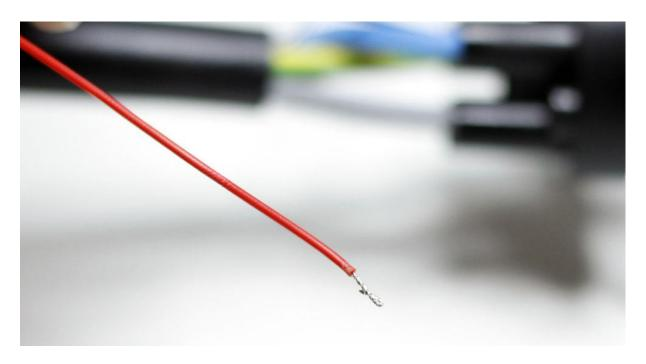
Slide a pice of shrinking sleeve over the small cable wires and crimp the small small terminals on the wires:
